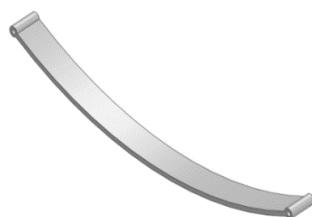
Figure 5. 3D modeling of mono leaf spring using SolidWorks CAD software.
