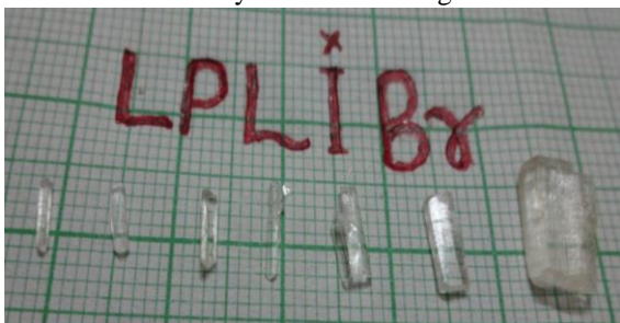
Figure 1. As grown single crystals of LPLBM from slow cooling technique Characterizations
